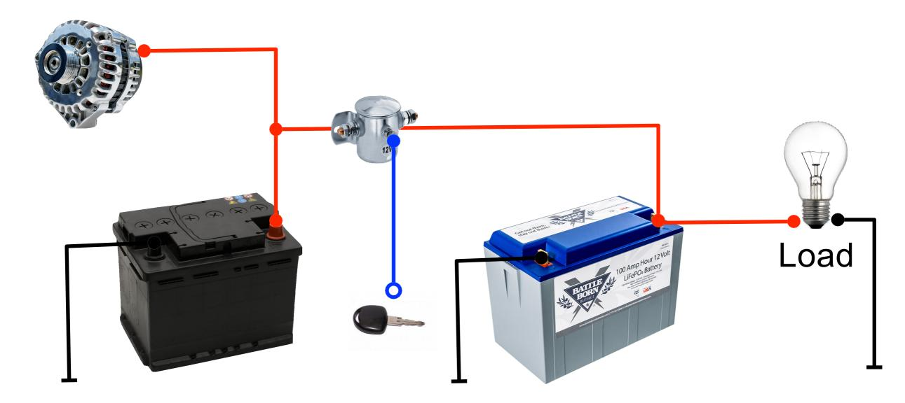
Back to the Future! This is probably the most classic dual battery set up. An ignition controlled switch means that the batteries are in parallel only when the engine is running.
